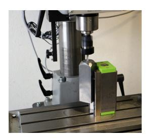
The MBX magnetic blocks have two opposite locking sides that could be concurrently activated. They are designed to lock parts on steel surfaces such as machines or assembly tables.
