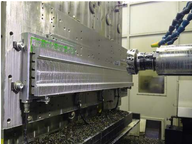
Milling on toolpaths, clamped in vertical tension on mobile pole extensions
